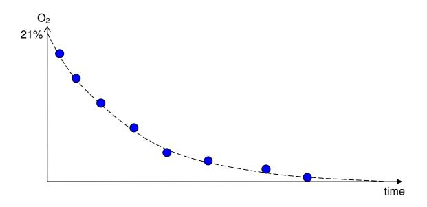
If the oxygen concentration is measured regularly until all oxygen has been consumed, a curve similar to the above can be outlined.
