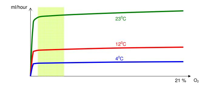
As shown above, it is important to consider temperatures when designing packaging. For this reason test tubes and subsequently test packages must be kept at the right temperature during tests. The right temperature is the highest temperature, at which the product is kept for a longer period during distribution.
