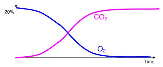
The figure shows the oxygen and carbon dioxide concentrations in packaging with fruit and vegetables.
