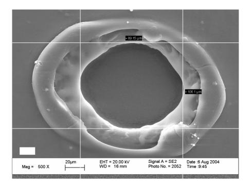
The ultimate solution for perforation plastic film is with a laser, but it is also the most expensive of the existing solutions, as it requires expensive specialist equipment. It is possible to make holes down to approx. 10  $\mu$ m thicknesses and up to 200  $\mu$ m. Laser perforation will typically make slightly oval holes. The advantage of laser perforation is that it is proportionately easy to control the size of the hole.
