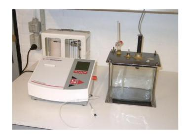
The picture shows a set-up with respiration vessel and an instrument which measures the oxygen and carbon dioxide contents of the container.
